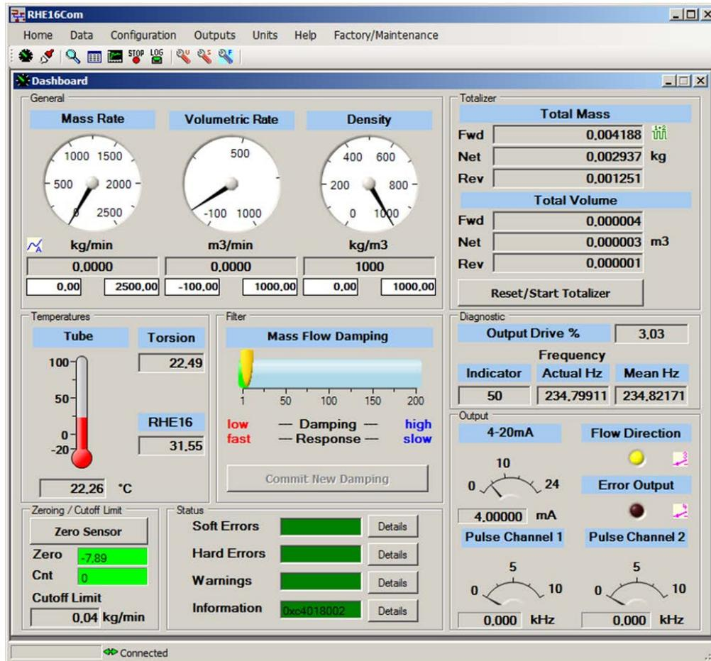
RHECom software is designed to ensure simple and expedient setup of the transmitter features and functions. The program operates on Windows™ based computers and has an intuitive user interface. Connection is via a standard USB port or the native RS485 connection of the transmitter. Communication between RHECom software and the transmitter uses MODBUS protocol.
